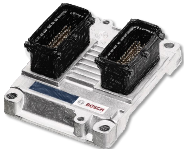
Bosch used hybrid die substrate on the Ferrari 360 ECUs’...
