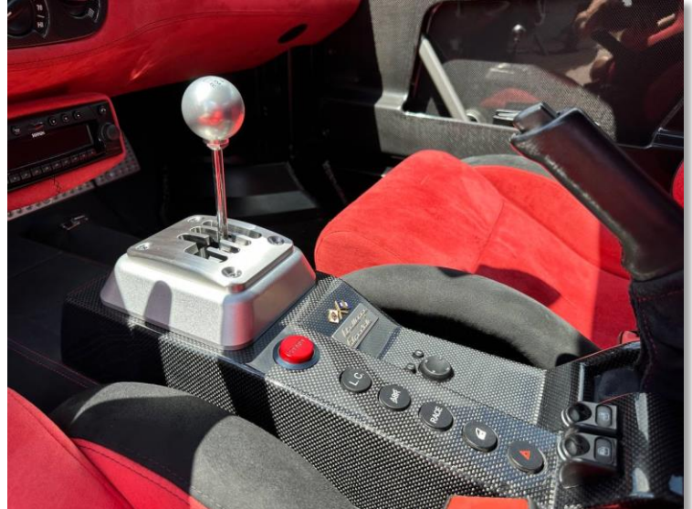
Challenge Stradale with a re-manufactured 'OEM Inspired' gated central tunnel for that factory look in Carbon exactly like the original F1 version.
