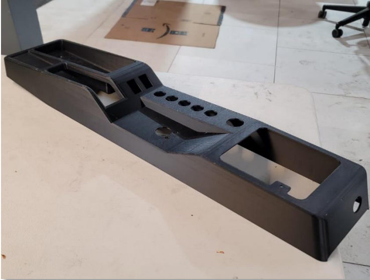
Rapid prototyped central tunnel replacement unit was 3D printed to quickly evaluate different designs before being productionized.
