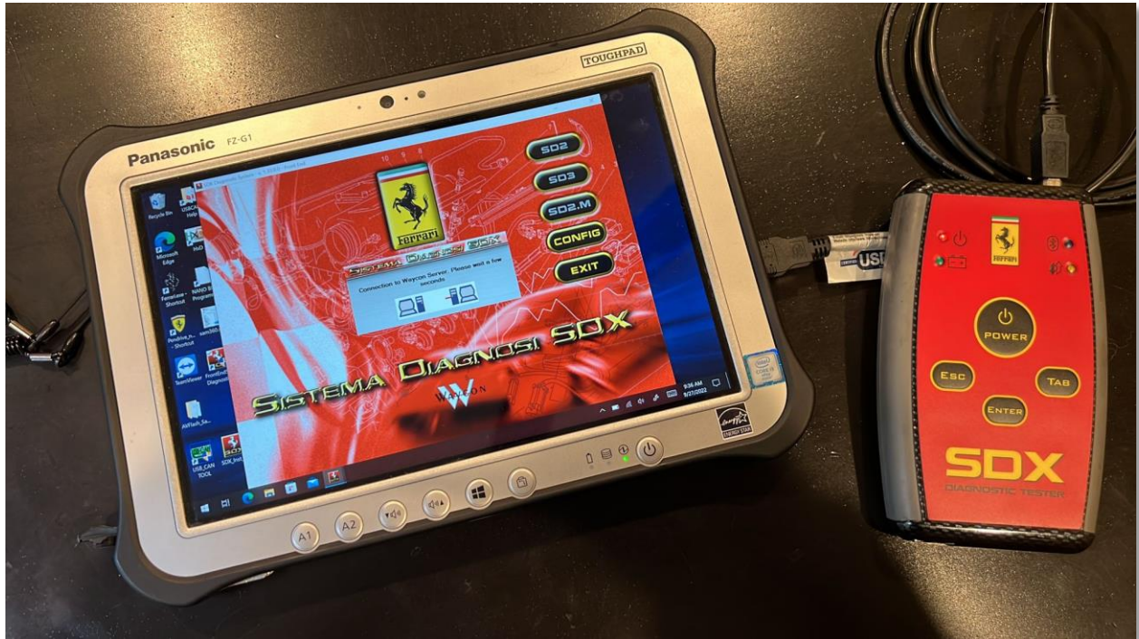
SDX software and VCI controller is vastly more capable than your typical generic scan tool and used by dealers and specialists alike
