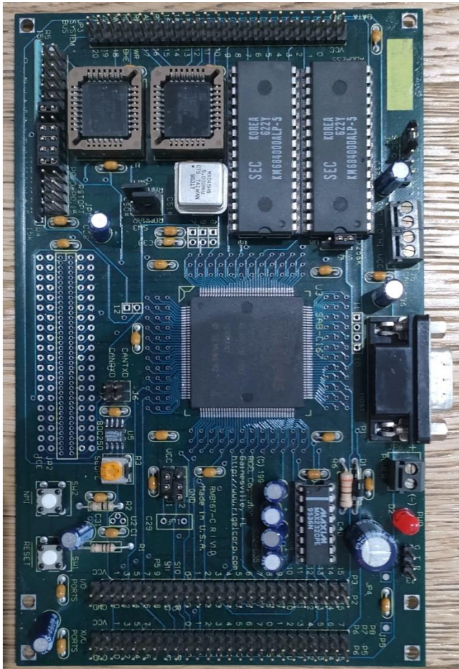
A 'Period' 1996 vintage Siemens C167 Reference Design board from Rigel Corp which allowed to get familiar with the hardware before designing your own.
